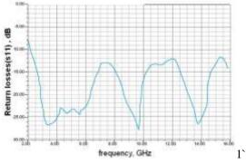
Fig. 1(b): s<sub>11</sub> versus frequency plot (BW is from 2.8GHz to 15 GHz).
