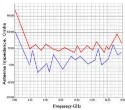
Fig. 1(c) : Antenna impedance versus frequency (real part  $\rightarrow$  red color and imaginary part  $\rightarrow$  blue color) of circular Planar UWB monopole Antenna.
